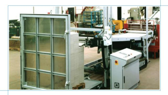
B-PAL is a device studied to palletize high volume production of pads, corrugated board, solid fiber board, padded board / press pan, acetate, foam and plastic materials with different thicknesses.
