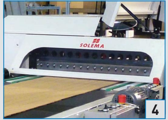
Crosscut is done by two superimposed blades that moving upwards (lower blade) and downwards (upper blade) cut the sheet crosswise. Cutting speed is set automatically and each time the blades open up, an impulse is given by the photocell to the drive, instructing to advance the sheet.
